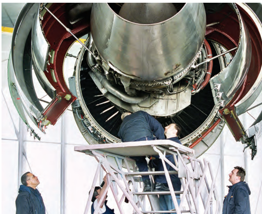
ABOVE: TROUBLESHOOTING A CF6-80C2 ENGINE. Image courtesy of Lufthansa Technik.
